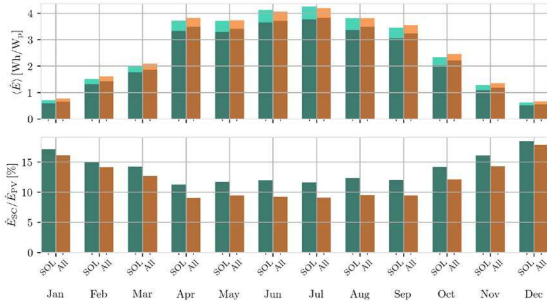
Figure 9-26. Monthly self-consumption derived with a stochastic bottom-up model for a German control area (TransnetBW) during 2018
