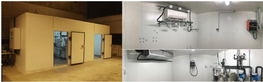
Figure 6: Test bench, outside view (left), cooled room (right, up), outside conditions (right, down)
