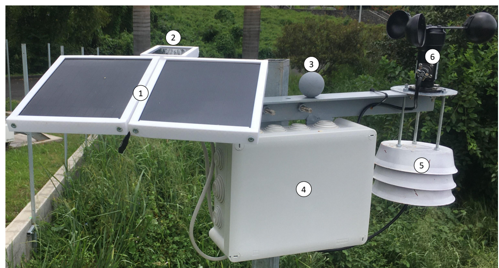
1: 6 W power supply; 2: low-cost pyranometer; 3: gray globe; 4: junction box for PCB and battery; 5: solar radiation shield for thermo-hygrometer; and 6: anemometer.
