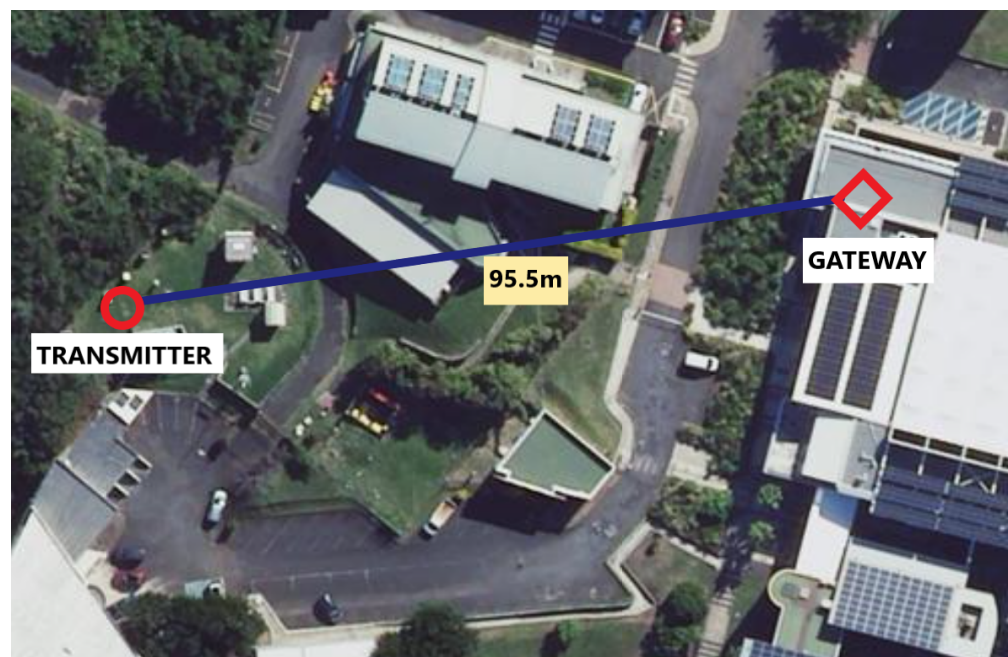
Figure 8. Aerial perspective of the in situ deployed LoRa devices at St Pierre, La Reunion.
