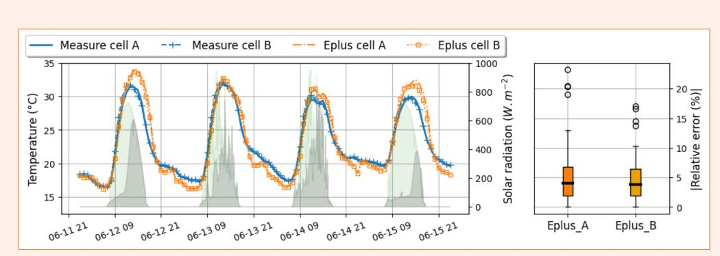
Figure 5: Simulation results for North wall without PCM
