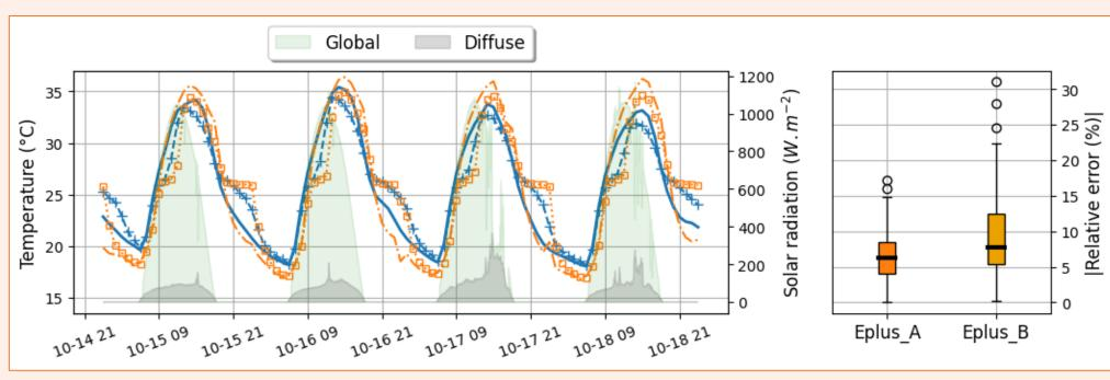
Figure 6: Simulation results for North wall with PCM
