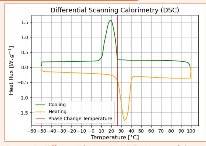
Figure 3: Differential Scanning Calorimetry of the PCM (5°C/min)
