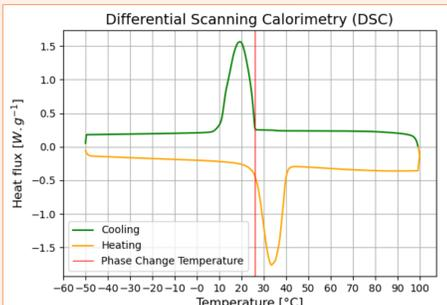
Figure 3: Differential Scanning Calorimetry of the PCM (5°C/min)
