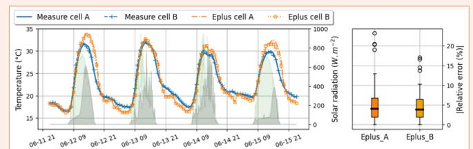
Figure 5: Simulation results for North wall without PCM
