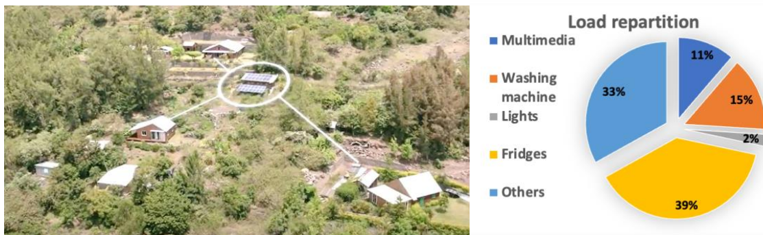
Fig. 2: Aerial view (Francou 2022) and repartition of electric load of the remote microgrid located in the Mafate cirque, La Reunion
