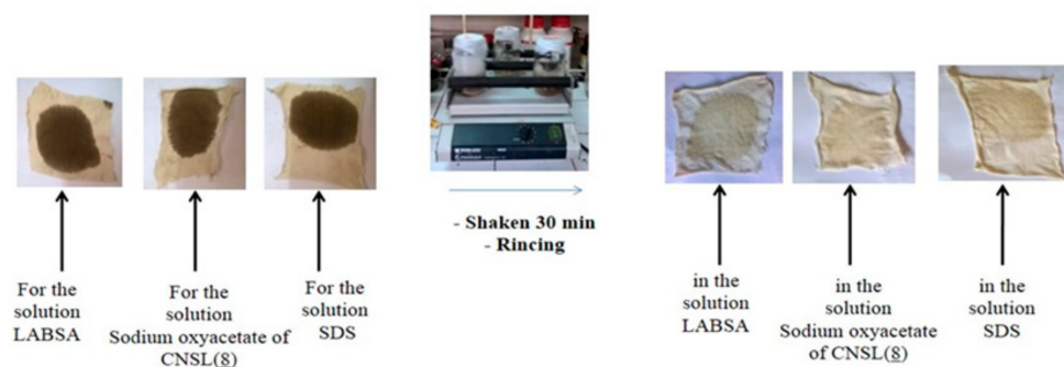
Figure 4. Detergent with LABSA, sodium oxyacetates of CNSL (8), and SDS.
