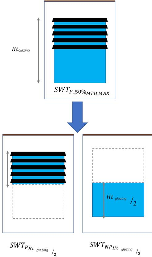
Figure 4: Methodology to calculate the  $C_m$  coefficient with 50 % of glazing shading
