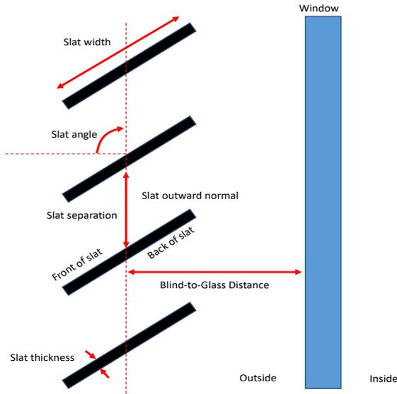
Figure 2: Lower configuration and parameters used in simulations
