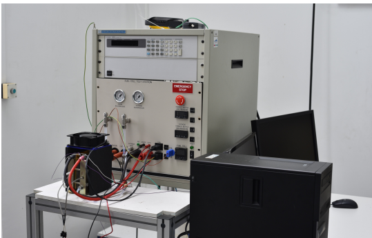
Figure 13. Laboratory test bench with its single cell
