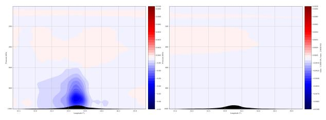
**Figure 12.** Specific humidity analysis increment on zonal section (51°3 E–55°3 E, 12°2 S) across TC center on 7 February 2019 02:00Z for SAR\_12km\_2ms (**left**) and NO\_SAR (**right**).
