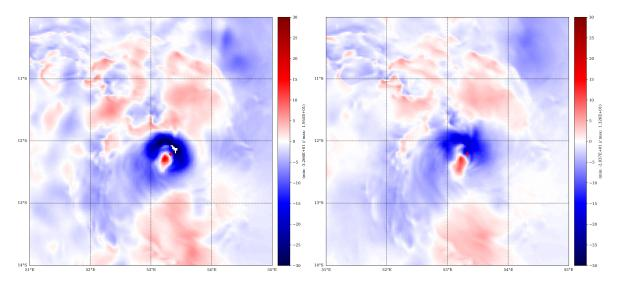
**Figure 19.** Analysis increments for surface wind speed with thinning of 5 km (**left**), 20 km (**right**) for SAR data assimilation. Units are  $m \cdot s^{-1}$ . Red cross is the estimated TC center position interpolated from TC position extracted from BT on 7 February 2019 00:00Z and 06:00Z.
