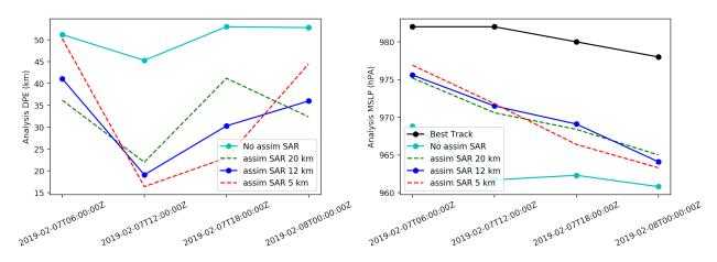
Figure 16. Evolution of DPE (left) and MSLP (right) in analyses of 7 February 2019 06:00,12:00, 18:00Z and 8 February 2019 00:00Z for NO\_SAR, SAR\_12km\_2ms, SAR\_5km\_2ms, SAR\_20km\_2ms.
