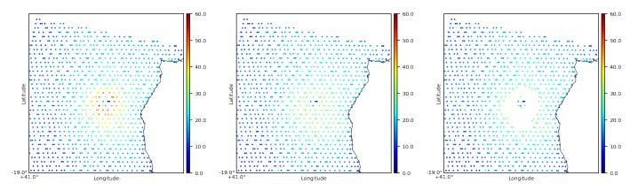
**Figure 25.** SAR wind speed observations assimilated within 51° E–55° E, 10° S–14° S with observations in experiments SAR\_12km\_2ms (**left**), SAR\_12km\_max30 (**middle**) and SAR\_12km\_no30 (**right**). Units are  $m \cdot s^{-1}$ .
