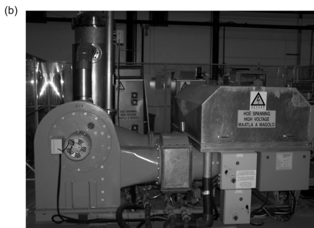
Fig. 1. Parasite LP experiment: (a) schematic layout of the kilowatt CO 2 laser chain developed at Pelindaba for the MLIS programme for isotope separation by laser. Amplifier 1 is a double-pass system, thus there are six amplification stages after the oscillator. (b) One laser in the Master Oscillator Power Amplitude (MOPA) chain (to give a sense of the size of the combined equipment), showing the gas circulating system with the laser head. Such an element can be configured to deliver 1 kW of average power and was used for the repeat CO 2 laser propulsion experiment.
