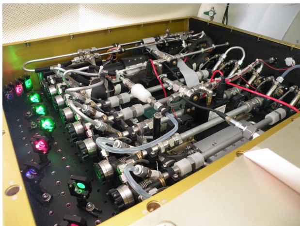
Figure A2. The eight separate ring-down cells in the CRD instrument.
