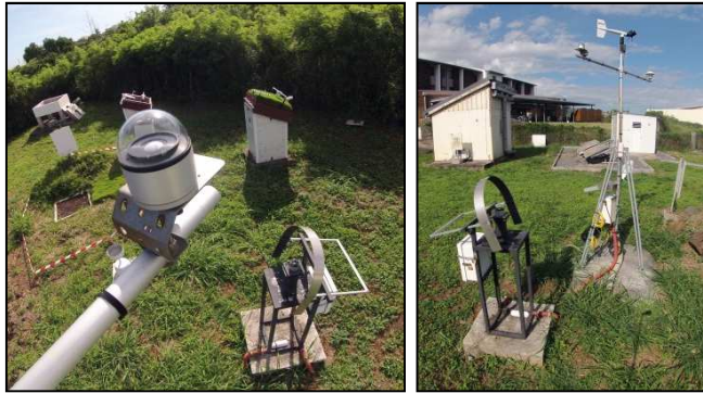
Figure 3: Outdoor luxmeters for global and diffuse illuminance
