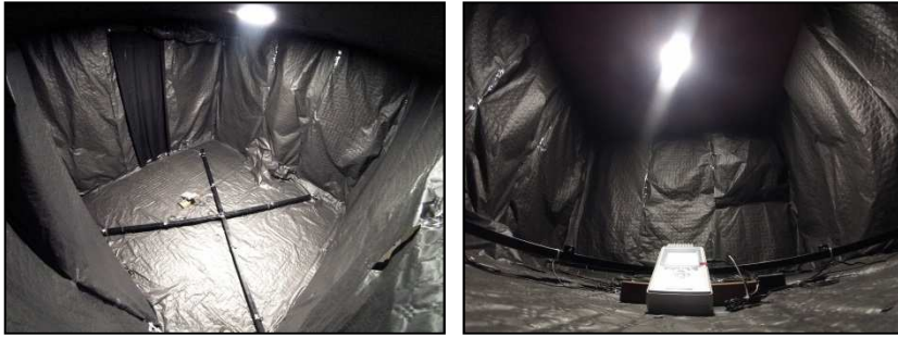
Figure 5: Experimental cell with black inner walls
