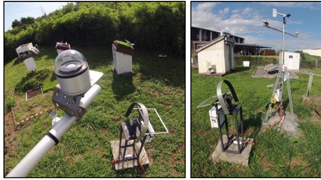
Figure 3: Outdoor luxmeters for global and diffuse illuminance
