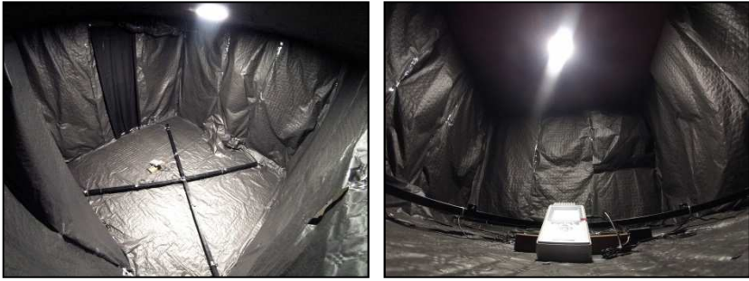
Figure 5: Experimental cell with black inner walls
