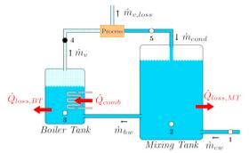
Fig. 1. Current heat supply system of the Sorélait-Danone firm.
