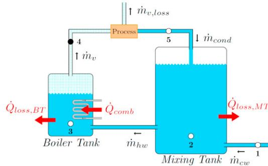
Fig. 1. Current heat supply system of the Sorélaït-Danone firm.
