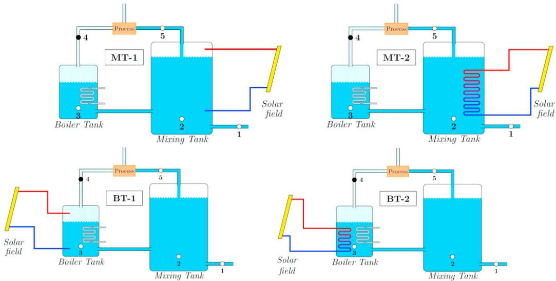
Fig. 4. Studied cases of solar heat integration into the current system – **MT-1**: direct integration into the mixing tank; **MT-2**: indirect integration into the mixing tank through an internal heat exchanger; **BT-1**: direct integration into the boiler tank; **BT-2**: indirect integration into the boiler tank through an internal heat exchanger
