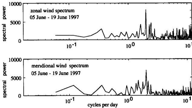
**Figure 2.** Spectrum of each of zonal and meridional wind components measured by ESRAD using spaced antenna technique applied to the PMSE between 05 June and 19 June 1997 for the height interval 84-86 km. 1-hour averaged winds are used with original radar height resolution 150 m, averaged over 13 gates.
