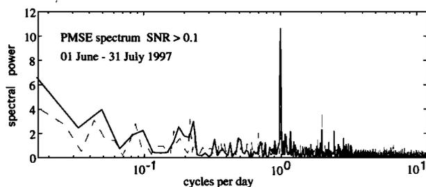
**Figure 1.** Spectrum of PMSE occurrence at ESRAD between 1 June and 31 July 1997. Occurrence is defined as SNR > -10 dB, and is based on one-hour average SNR for the height interval 84-86 km: solid line corresponds to measurements with 150 m original radar resolution, dashed line to 600 m.
