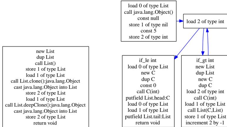
**Fig. 2.** The Java bytecode of `main` and of the empty constructor of `List` in Fig. 1.
