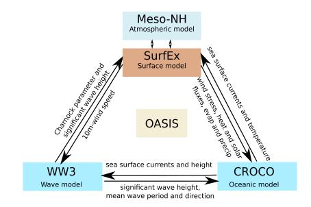
Figure 3. Schematic diagram of the coupling system. Fields exchanged among the atmospheric, wave, and oceanic models are also presented. All the parameters are exchanged at 10 min intervals.
