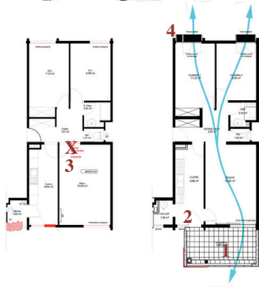
Figure 7: Plan view of a representative unit before (left) and after (right) retrofitting so as to enhance natural ventilation by (1) creating covered exterior verandas, (2) enlarging the openings, (3) removing non-loadbearing elements and (4) adding louvered shutters on solar exposed windows. Design: Endémik.
