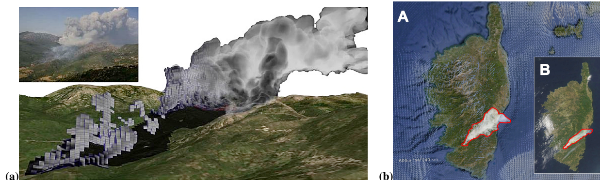
Figure 11. Simulated smoke tracer on 23 July 2009 (a) in the 50 m resolution domain compared to the plume's photograph (at the top left) and (b) in the 600 m resolution domain highlighted in red (A) at 15:00 UTC compared to the MODIS image (B) of Corsica at 14:50 UTC.
