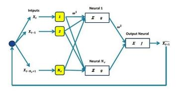
Figure 2: Multilayer Perceptron architecture
