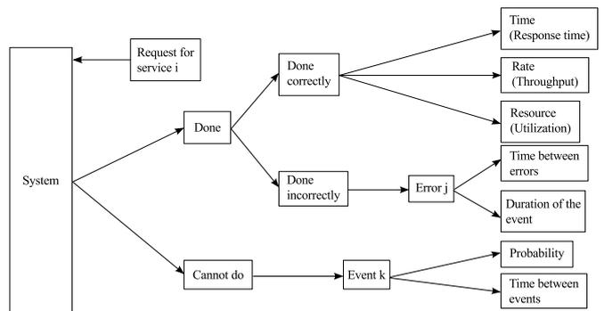
Fig. 3: Functioning of a request system
