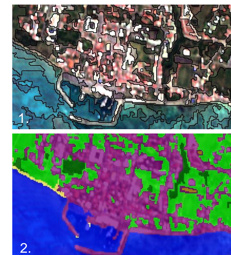
The two stages of object-based image analysis 1. segmentation of the satellite image 2. hierarchical classification
