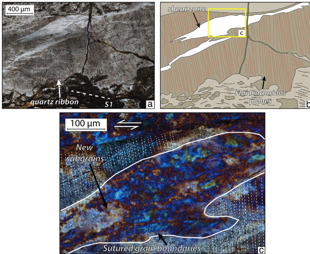
**Fig. 8.** a–b) Shear band cutting across a quartz ribbon. The shear band is characterized by a low density in fluid inclusions with respect to the surrounding quartz, apparent in the color contrast. Grain size reduction is observed inside the shear band. The small grains are characterized by sutured boundaries. a) Optical microscope transmitted light, b) with cross nicols and wave plate.
