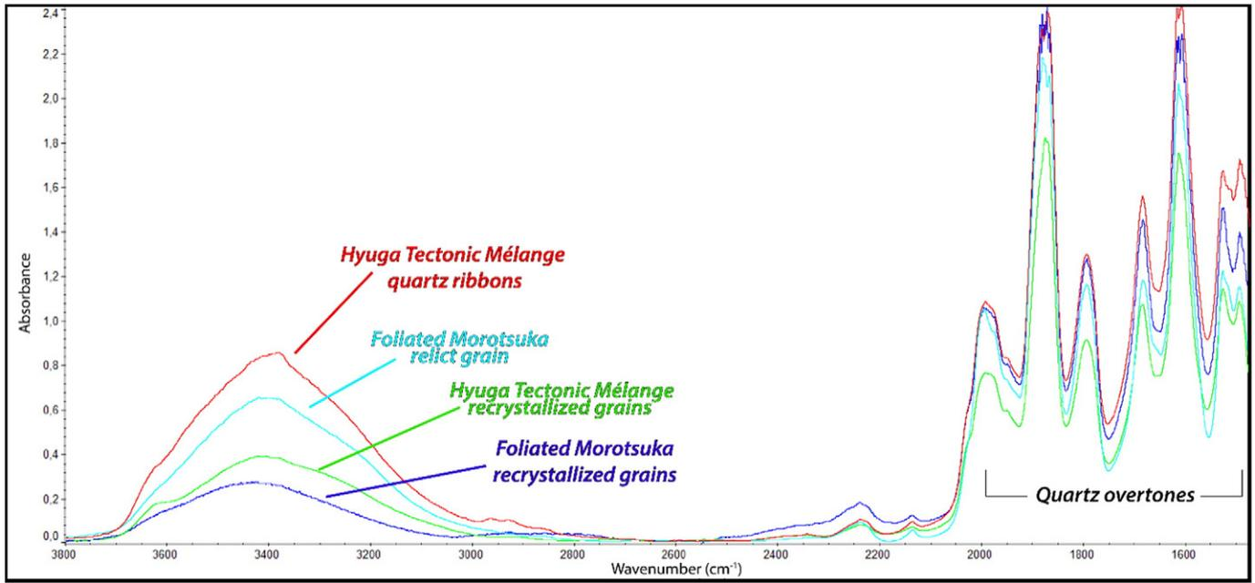
**Fig. 13.** Characteristic FTIR spectra for quartz ribbons (red) and recrystallized grains in shear bands (green) in Hyuga Tectonic Mélange and relict (cyan) and recrystallized grains (blue) in quartz veins in Foliated Morotsuka. Si—O vibrations are the 7 peaks from 2000 to 1400  $\text{cm}^{-1}$ .
