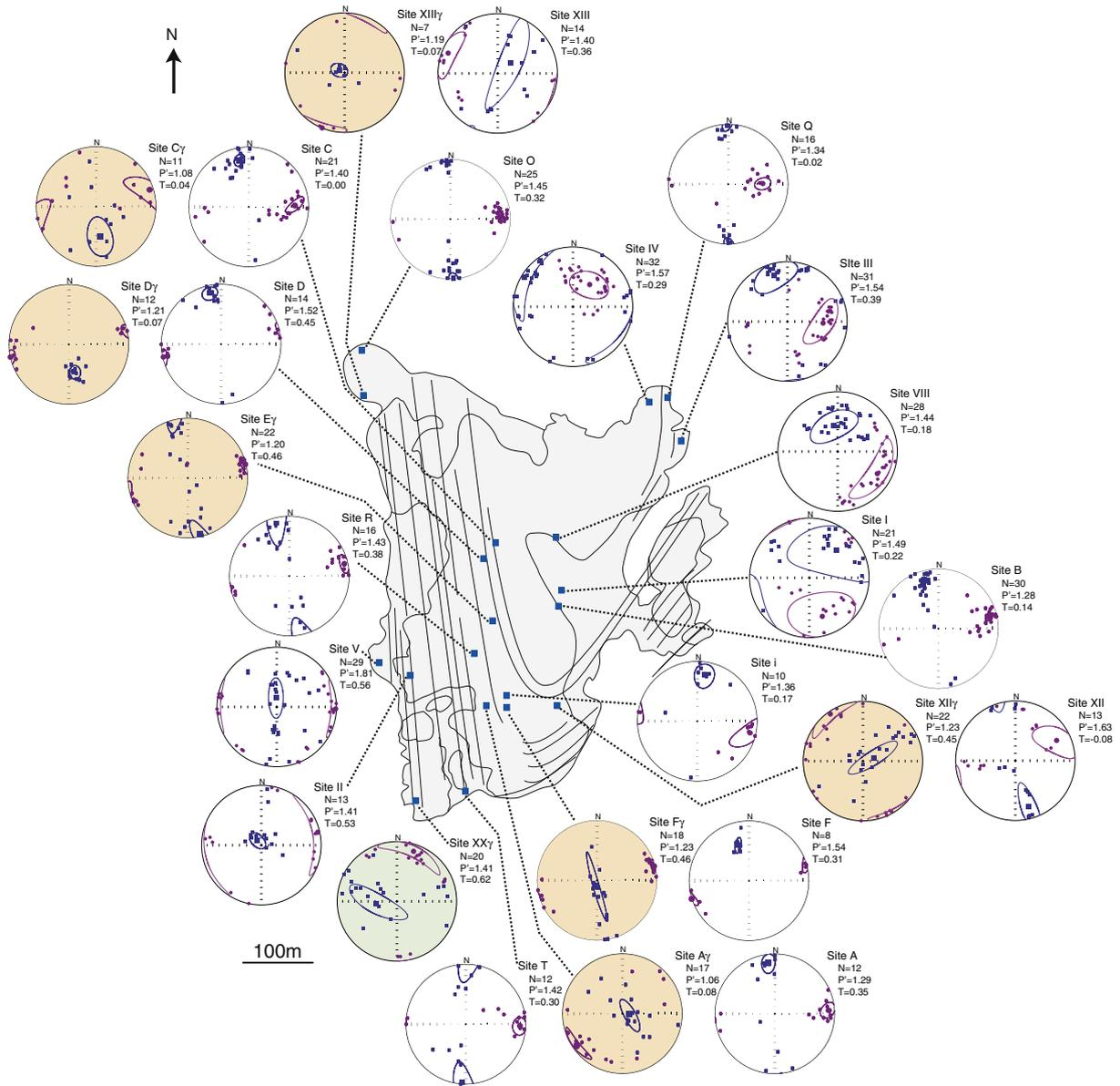
**Fig. 10.** Projection of AMS data of each site of Pétrels Island. Distribution of maximum axes ( $K_1$ ; blue squares) and minimum axes ( $K_3$ ; violet circles) with confidence ellipses is in lower hemisphere equal area projection. White, salmon and green colours of stereonets background represent the AMS projections of gneisses, granitic dykes and anatexites, respectively.
