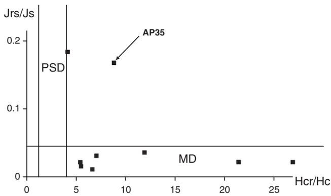
**Fig. 8.** Ratios of hysteresis parameters (Day et al., 1977):  $J_{rs}/J_s$  ( $J_{rs}$ : remanence at saturation;  $J_s$ : magnetization at saturation) as a function of  $H_{cr}/H_c$  ( $H_{cr}$ : remanent coercive force;  $H_c$ : coercive force). Areas for Multi-Domain (MD) and Pseudo Single Domain (PSD) grain size for pure magnetite.
