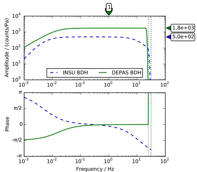
Figure 5. Bode plot of the total instrument responses  $G(f)$  as defined in Eq. (A2) of a DEPAS HighTechInc HTI-PCA04/ULF hydrophone (solid green, station RR26), and of an INSU differential pressure gauge (dashed blue, RR28). The nominal corner period is 100 s for DEPAS instruments and 500 s for INSU instruments. Dotted lines mark the Nyquist frequencies (see above).
