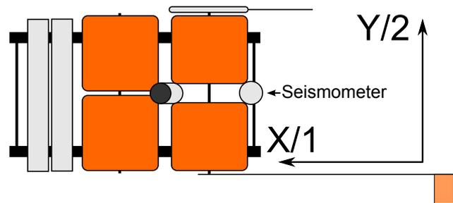
**Figure 3.** Sketch of a LOBSTER frame with the orientation of the horizontal seismometer channels. The X channel is oriented along the long axis of the LOBSTER, the Y channel 90° clockwise of it. Positive values in the seismogram correspond to movement in the direction of the arrow. For the vertical (Z) channel, positive values correspond to upward movement. In the RESIF data archive, the X channel is stored as BH1, the Y channel as BH2 and the Z channel as BHZ.
