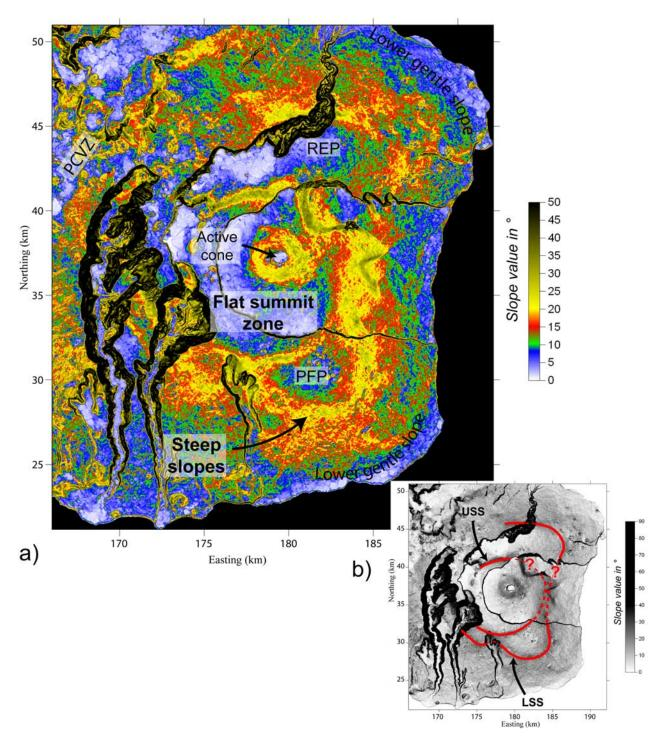
**Figure 3.** (a) Slope map of PdF showing the variable slopes on the volcano flanks. PFP, Piton de Fourche Plateau; REP, Rivière de l'Est Plateau; PCVZ, Plaine des Cafres Volcanic Zone. (b) Gray scale slope image with location of the upper and lower steep slope zones highlighted in red (USS and LSS) characterized by slope values ranging between 20° and 30°. Coordinates are in Gauss Laborde Réunion.
