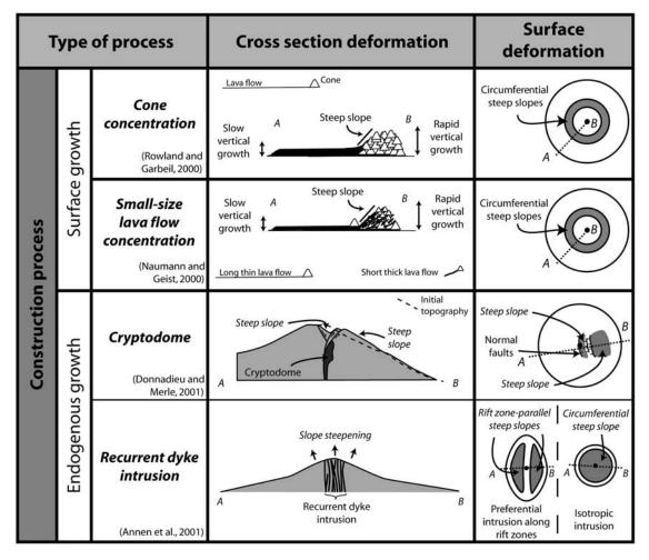
Figure 9. Construction processes able to develop steep slopes in basalt shield volcanoes.
