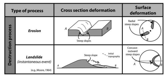
Figure 10. Destruction processes able to develop steep slopes in basalt shield volcanoes.
