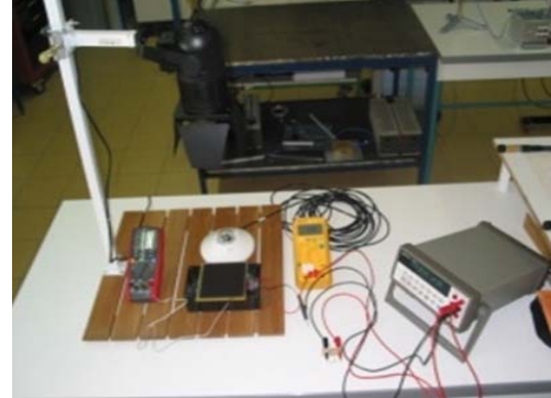
Figure10. Experimental PVcell test bench
