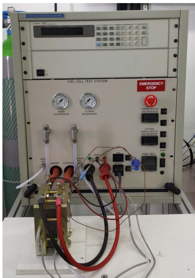
Figure 1. Fuel cell test station.
