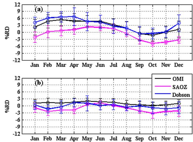
**Figure 5.** Monthly distribution of relative differences recorded between IASI and the other instruments (OMI SAOZ and Dobson): (a) from June 2008 to August 2010 and (b) from September 2010 to December 2012. The error bar is the standard deviation associated with the monthly mean distribution.
