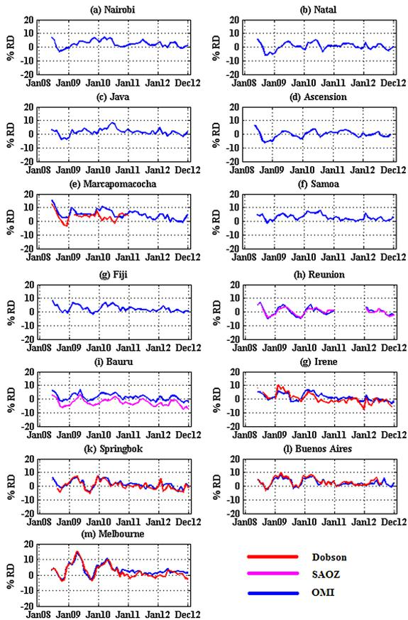
**Figure 4.** Monthly relative differences (% RD) of TCO observed from June 2008 to December 2012 between IASI and the other instruments (OMI (13 stations), Dobson (five stations) and SAOZ (two stations)).
